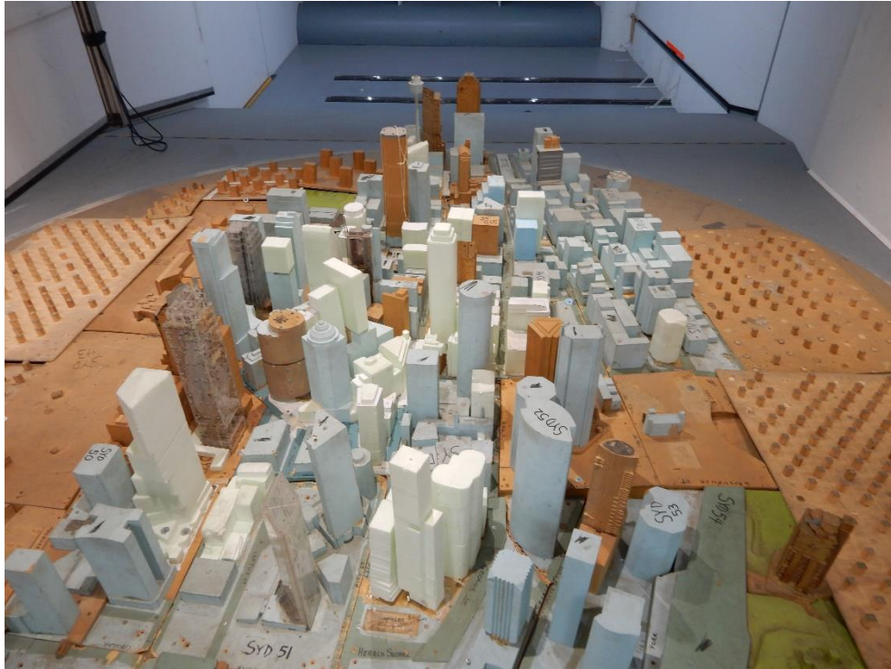
Figure 3 – View from the north of the 1/400 scale Proposed Configuration model of the 15-23 Hunter Street and 105-107 Pitt Street, Sydney in the wind tunnel.
