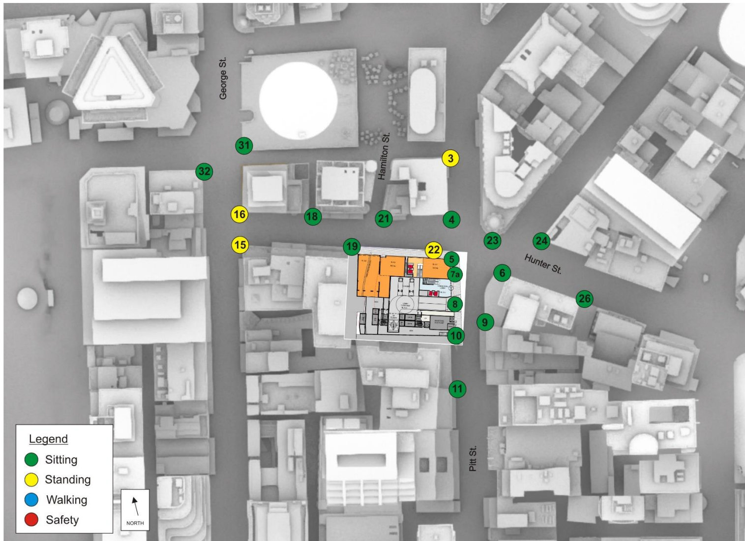
Figure 6 – Summary of ground level wind conditions for the Existing Configuration for 360° of wind direction.
